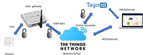
Data Logging Architecture Through Own Gateway
